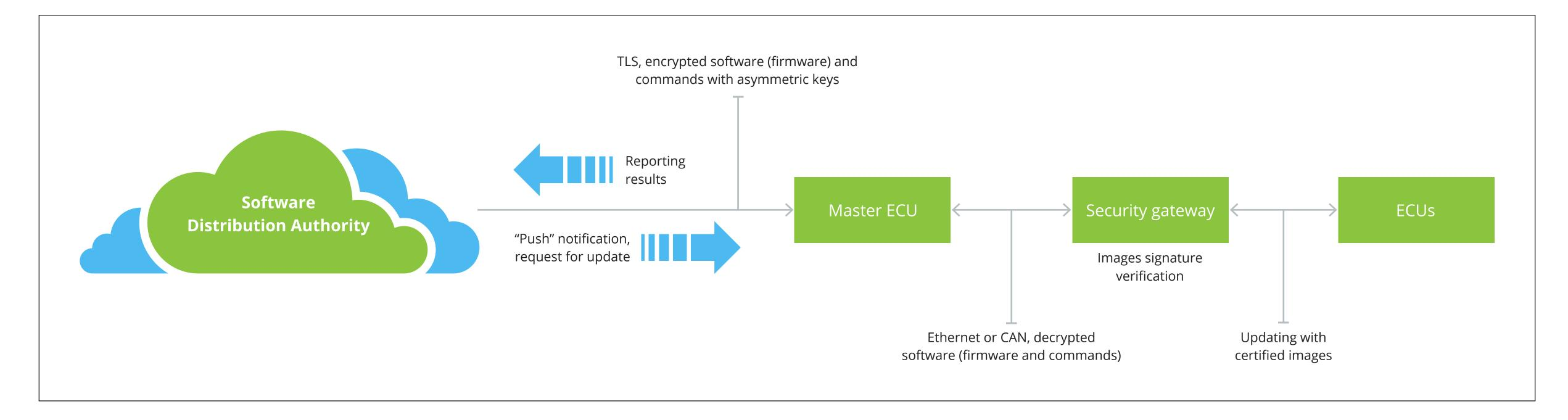
To ensure firmware installation regardless of disruptive factors, the software must be fully downloaded, the vehicle must be parked and the engine turned off. A Special Diagnosis manager is introduced as an extension to verify that the newly updated software operates as expected. It can also initiate rollback procedure to the previous software version.
